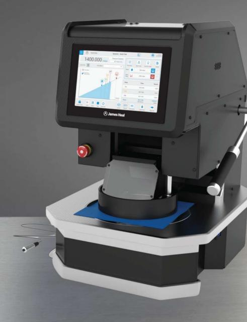
HydroView is used to measure the penetration of water through products including protective gloves, diving dry suits, winter sports apparel, fishing waders, roofing, tenting and ground sheets and more.
